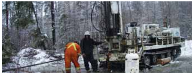
GEOTECHNICAL SOIL DRILLING AT MAKWA.
