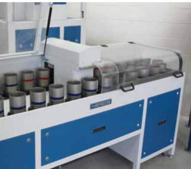
AUTOMATED PULVERIZER UNIT IN THUNDER BAY, ONTARIO.
