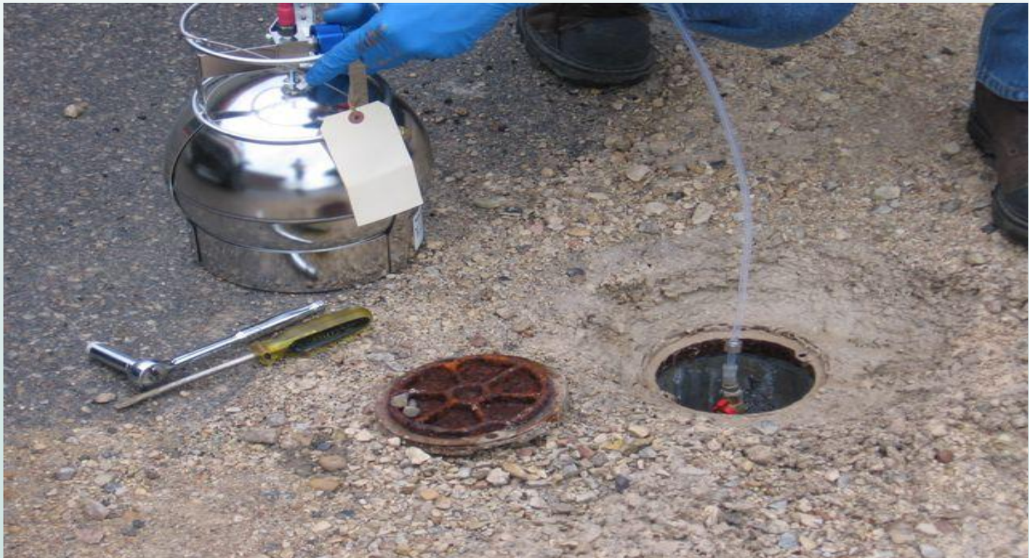
Vapour sampling with a Summa bottle
