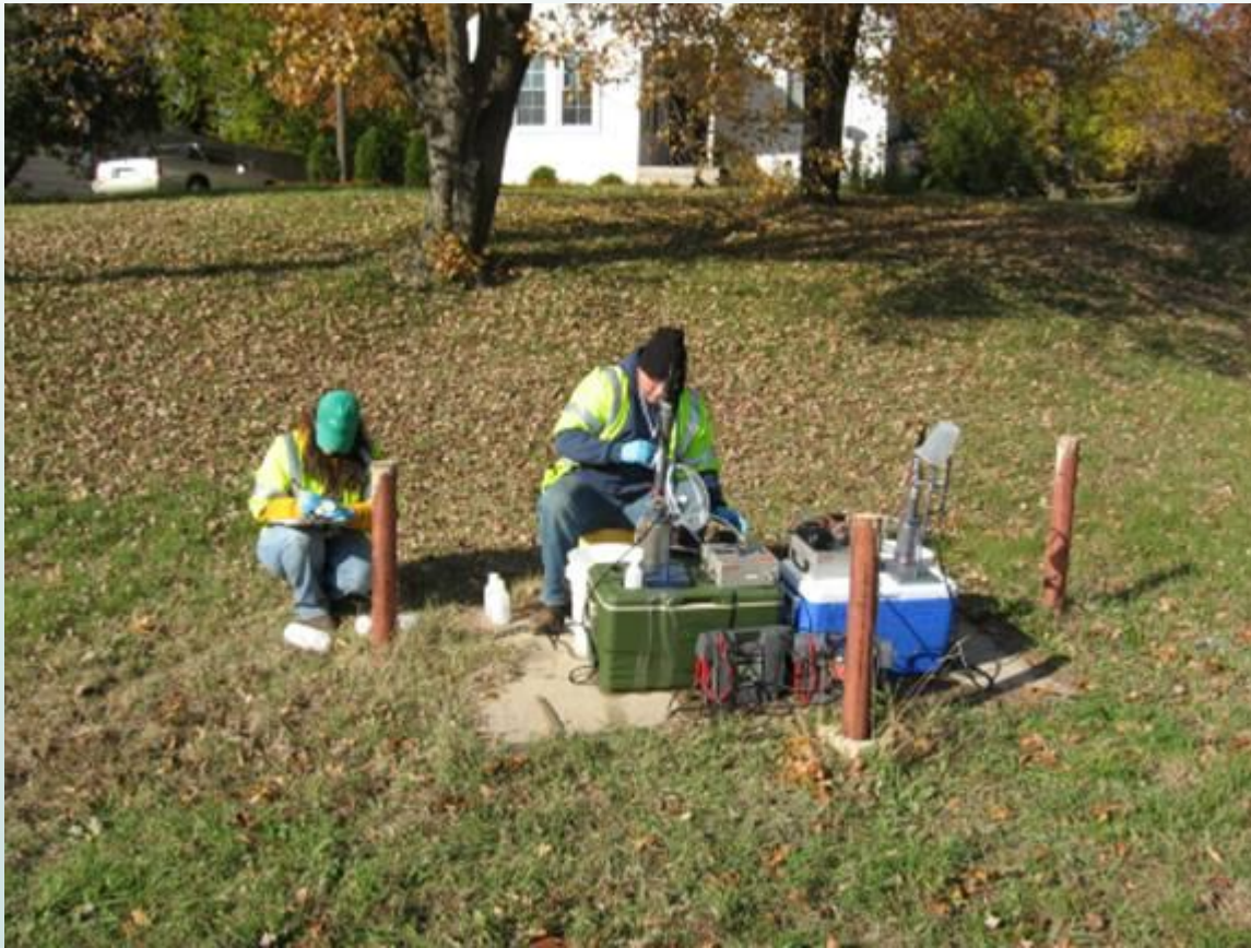
Low flow groundwater sampling
